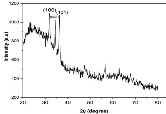
Fig. 1 XRD pattern of ZnO thin film deposited at 50<sup>0</sup>C
