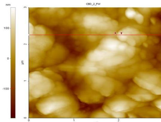
Fig. 2 The AFM image of the film of ZnO thin film deposited at 50<sup>0</sup>C
